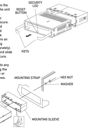
TYPICAL FRONT-LOAD DIN MOUNTING METHOD
